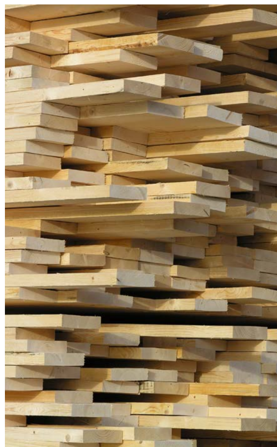
Boards for the production of CLT.
