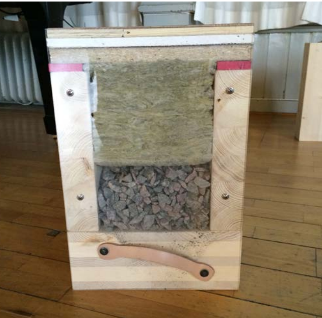
Example of floor structure.
