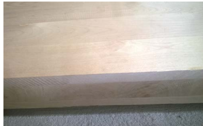
3-layer CLT panel made from birch.
