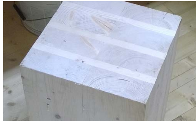
7-layer CLT block made from spruce.
